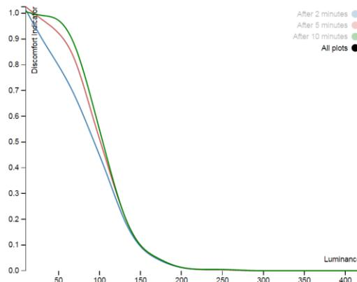
**Figure 3** Temporal weighted discomfort indicator (the three lines represent occupant discomfort after 2, 5, 10 minutes at the given luminance).
