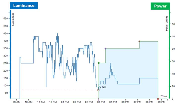
**Figure 1** (Indoor Luminance Levels (volatil line) vs Manual Control Actions (step-wise line).
