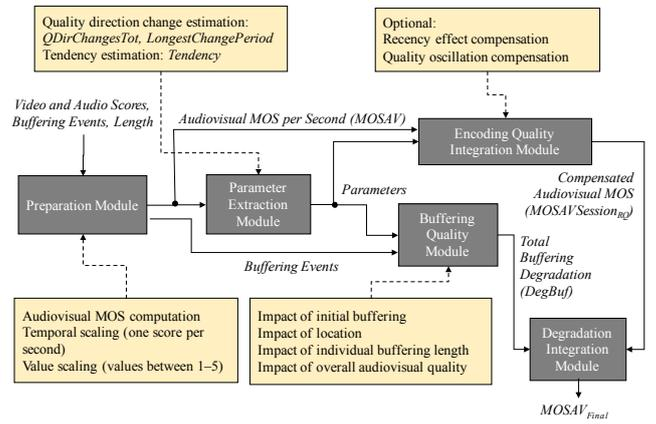
Fig. 1. Block diagram of the proposed model. Light boxes indicate steps inside modules.
