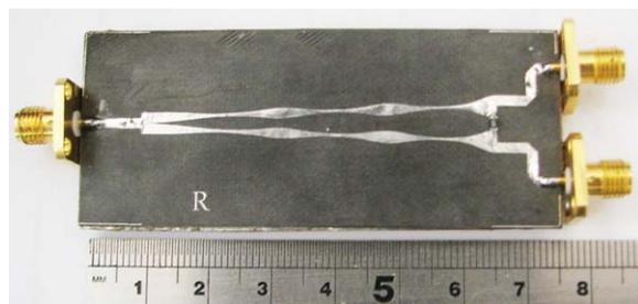
**Figure 6** The photo of the fabricated power divider of [1, 2.8, 4.5] GHz. [Color figure can be viewed in the online issue, which is available at [wileyonlinelibrary.com](http://wileyonlinelibrary.com).]
