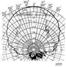
Fig. 2 E-plane radiation pattern of DRLWA
