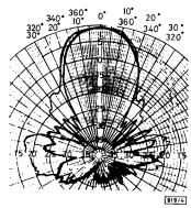
Fig. 4 Radiation pattern of DRLWA with dielectric overlays
