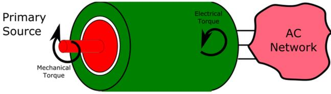
Figure 1: Simplified diagram of a synchronous machine directly connected to an AC system
