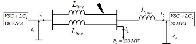
Figure 3: Diagram of the test system
