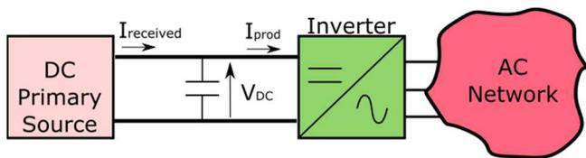
Figure 2: Simplified diagram of a PE-interfaced generating unit
