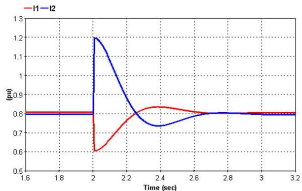
Figure 4: Currents injected by the converters
