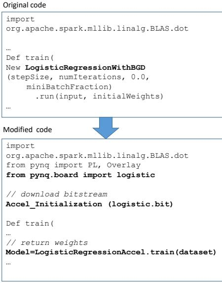
Fig. 2. Original and modified code for the logistic regression example
