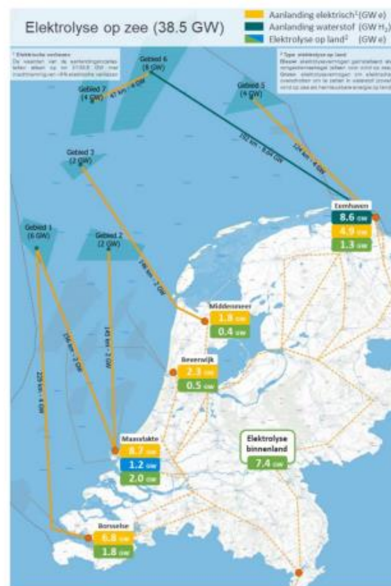
Figure 29 – Landfall scenario including offshore coupled electrolysis, onshore coupled electrolysis and grid-integrated electrolysis, based on national steering [63]
