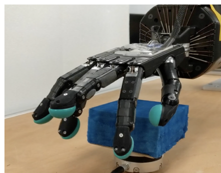
Figure 7. Gentle object manipulation with an anthropomorphic robotic hand [84].
