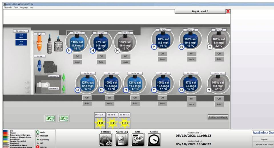
Figure 2: VIGO representation of probes and tanks in experimental system
