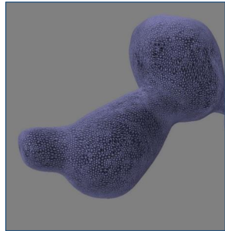
Figure 5: A close-up of what the mesh model looks like after the application has generated polygons from the point cloud.
