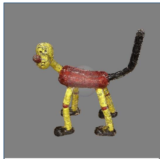
Figure 4: The toy dog has several small holes in its body (including in its face), which shows that the application has not found any reference points in those areas.
