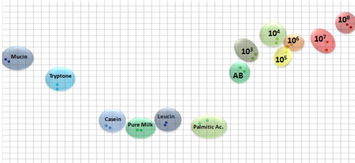
Figure 5. IDMAP plot for the Electrical Impedance Spectra from interferences and milk solution in PBS and S. aureus antibody (AB).
