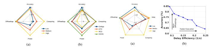
Fig. 7: Comparison of different key metrics (normalized): (a) On-Algo for low, medium and high traffic load. (b) Algorithm comparison for high load in scenario 2.
