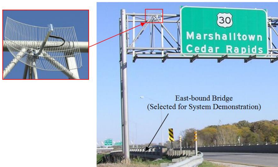
Figure 6 – Wireless communication equipment installed at the west end of the bridge.
