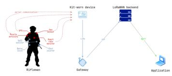
Figure 2: Soldier wearable high-level architecture
