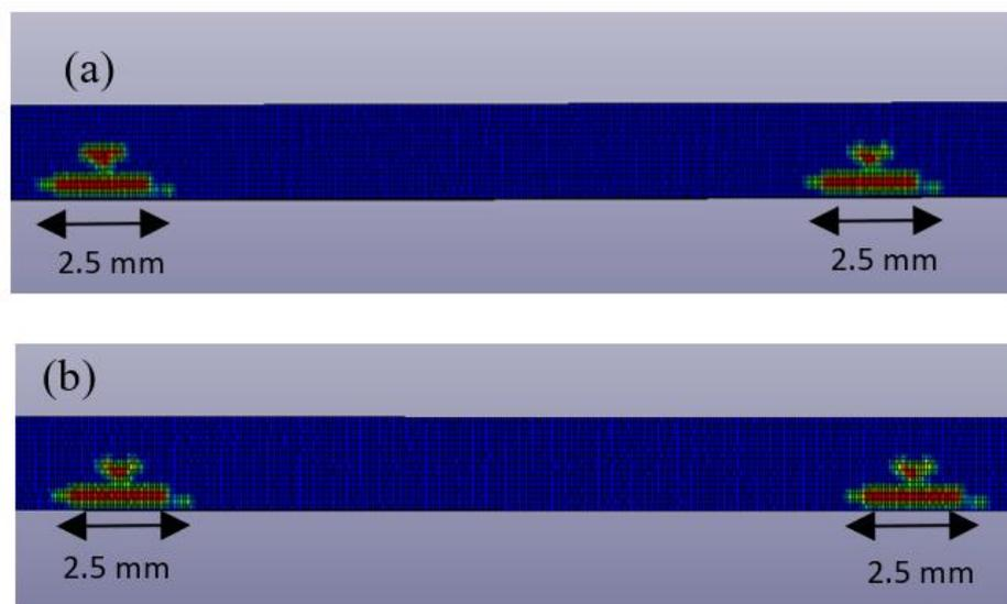
**Figure 7.** Damage pattern comparison, (a) single model, (b) multi-step model
