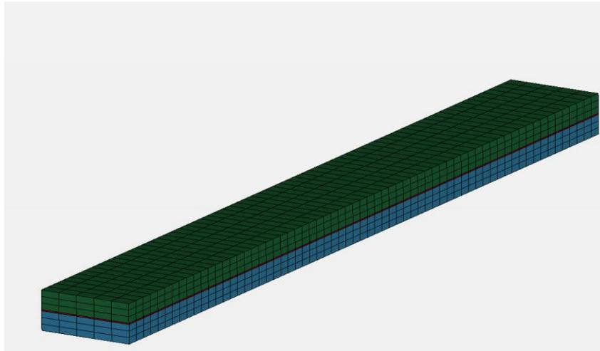
**Figure 3.** DCB model for Mode I simulation
