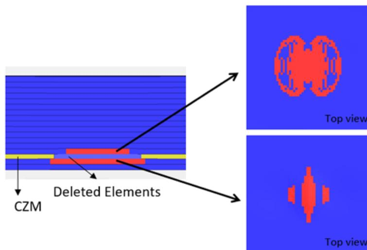
**Figure 10.** Delaminations caused by laser shock.
