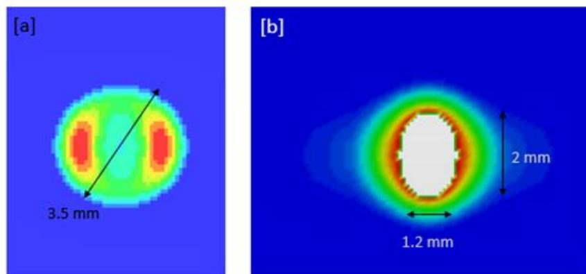
**Figure 9.** CZM at the loading spot, after the 1<sup>st</sup> load [a], after the 2<sup>nd</sup> load [b].
