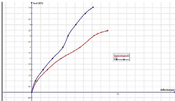
Figure-2: Test for point bends Deflection vs. Load for M30 Concrete
