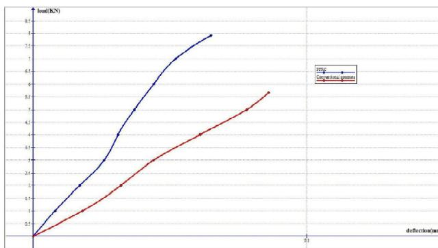
Figure-3: Point bend test for M35 concrete: Load vs. Deflection
