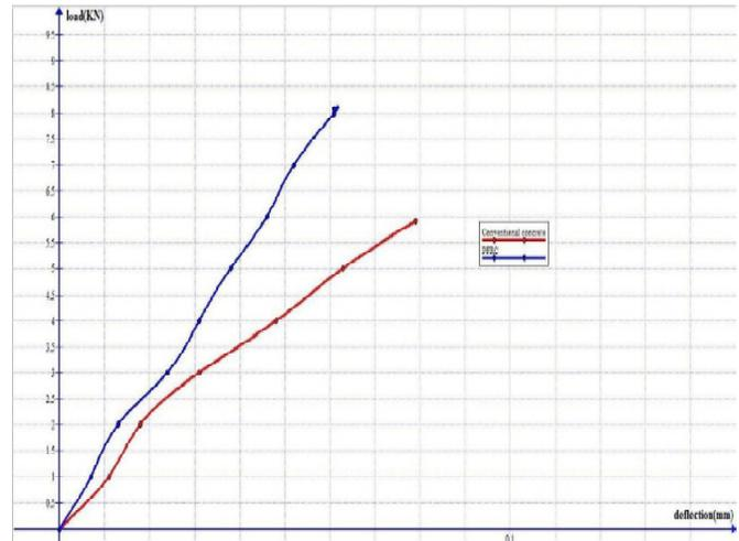
Figure-4: Point bend test for M40 concrete: Load vs. Deflection
