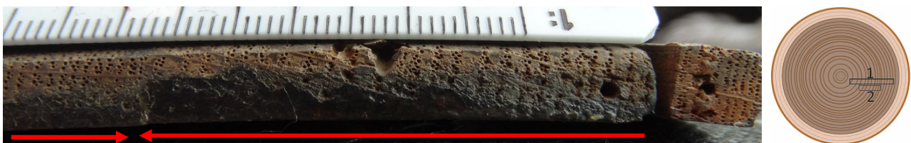
Figure 3. Detail of the joint between the two boards on the right-hand side of the panel (Board 1 is on the left). The semi-tangential processing, as illustrated in the diagram, can be observed. A 3 mm line was cleaned with scalpel blades to enable the accurate measurement of the tree-ring widths. The arrows indicate the growth direction (photo and diagram: M. Domínguez-Delmás).
