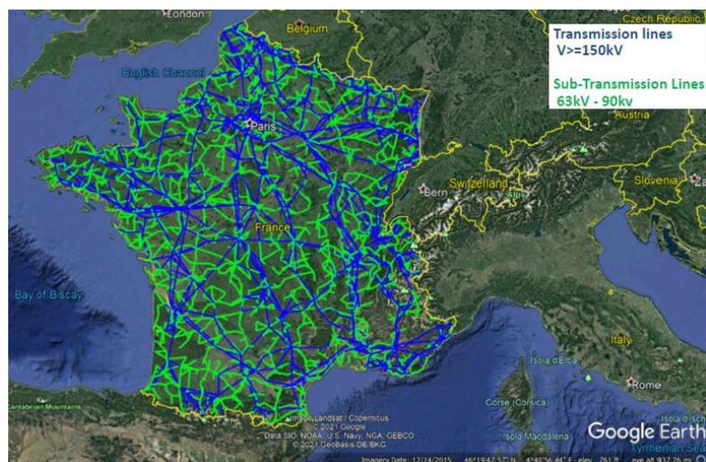
Figure 5 : French Transmission and Sub-Transmission Lines
