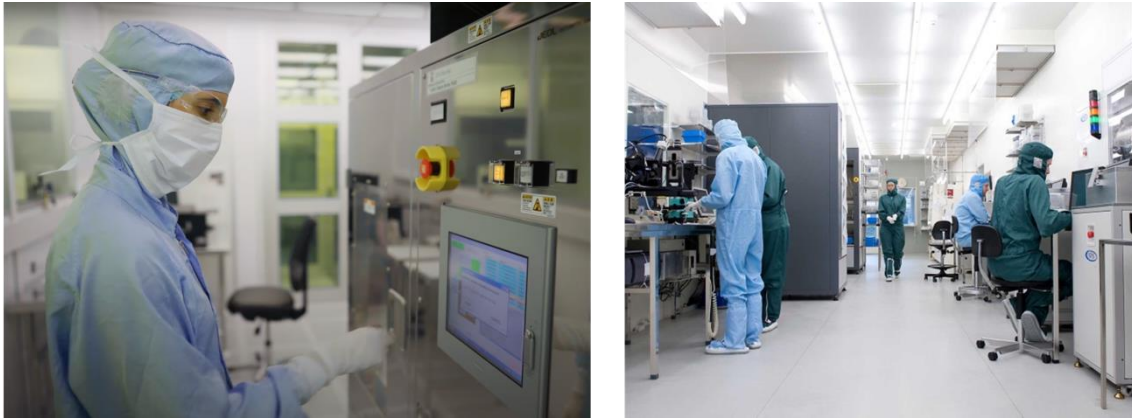
Figure 1 – Facilities at DTU Nanolab. (Left) Cleanroom user operating the Jeol JBX-9500-FS electron beam writer inside the Nanolab cleanroom. (Right) Several cleanroom users in protective suits inside the Nanolab cleanroom. Images courtesy of DTU Nanolab.
