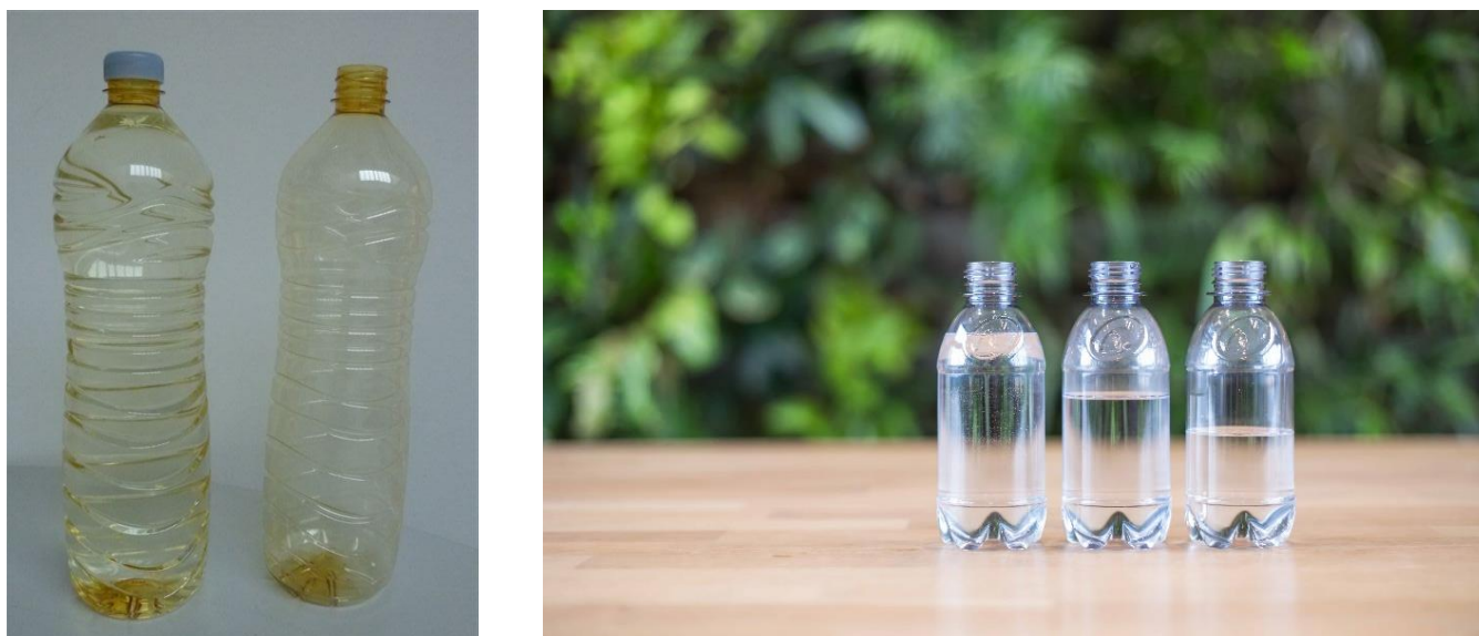
Figure 3. One of the first “golden” PEF bottles made ( left ) and typical examples of current fully transparent small size PEF bottles ( right ).
