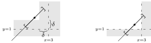
Fig. 2. The conservative- (left) and excess semantics (right) for a transition guarded with x \leq 3 \wedge y \geq 1 . The grey area corresponds to forbidden delays, the bullet corresponds to the choice of Controller, and the segment indicates the possible choices for Perturbator.
