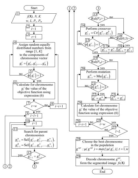
Fig. 1. The main stages of the method of segmentation of camouflaged military equipment in images from space surveillance systems using a genetic algorithm
