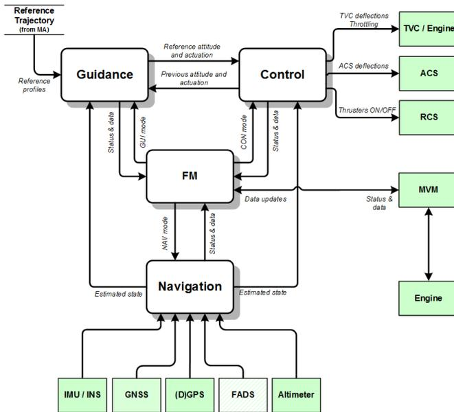
Figure 3 RETALT1 recovery GNC functional architecture
