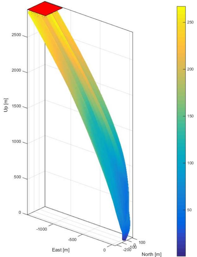
Figure 13 Trajectory path during the powered descent and landing phase
