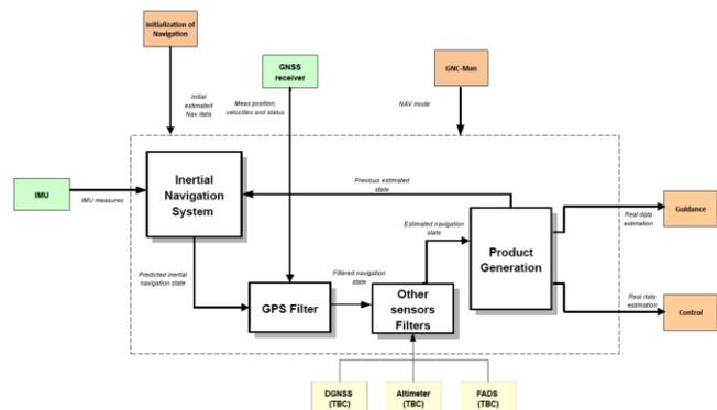
Figure 5 RETALT Navigation functional architecture
