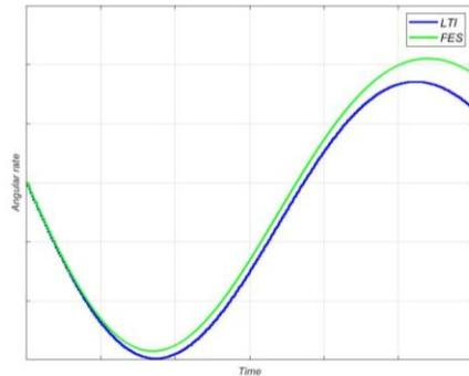
Figure 8 FES and LTI models comparison of open-loop response to a step of fin deflection at a specific operating point
