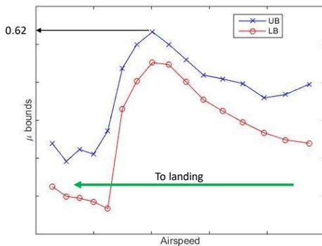
Figure 10 Structured singular value behavior along trajectory
