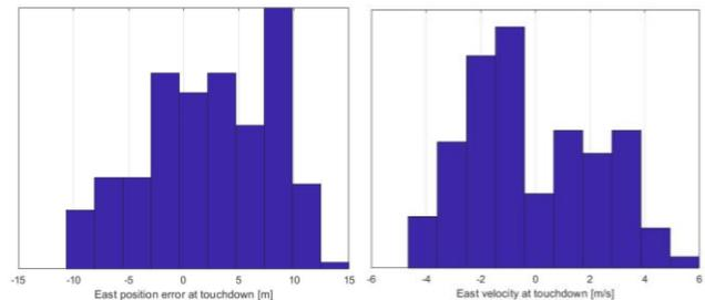
Figure 14 Statistics of position and velocity errors at touchdown
