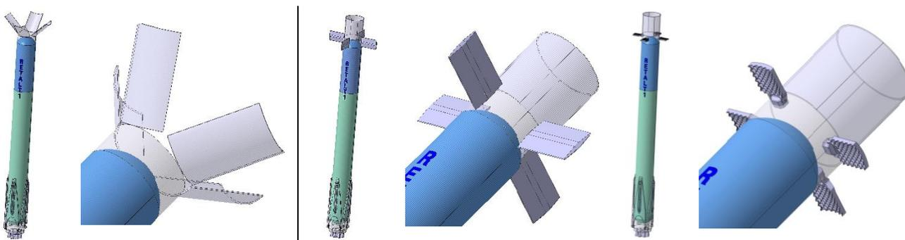
**Figure 3 RETALT1 ACS configurations: interstage petals (left), planar fins (center), and grid fins (right) [3]**
