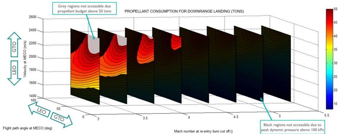
Figure 5 End-2-end propellant budget as function of conditions at MECO, RETALT1 PF configuration, DRL
