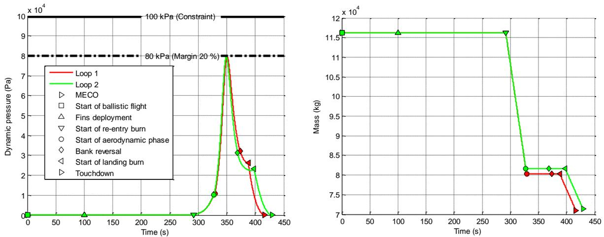
Figure 9 Dynamic pressure (left) and total mass profile for the DRL (R1 B) scenario
