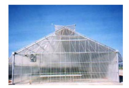
Figure 3.6 Glass or rigid plastic cladding, used in temperate climates
