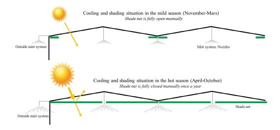
Figure 5.24 Design of the recommended nethouse
