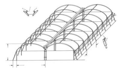
Figure 3.14 Round-arched greenhouse with sloped sidewalls
