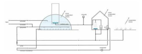
Figure 5.10 A closed water cycle between a closed greenhouse and an urban area
