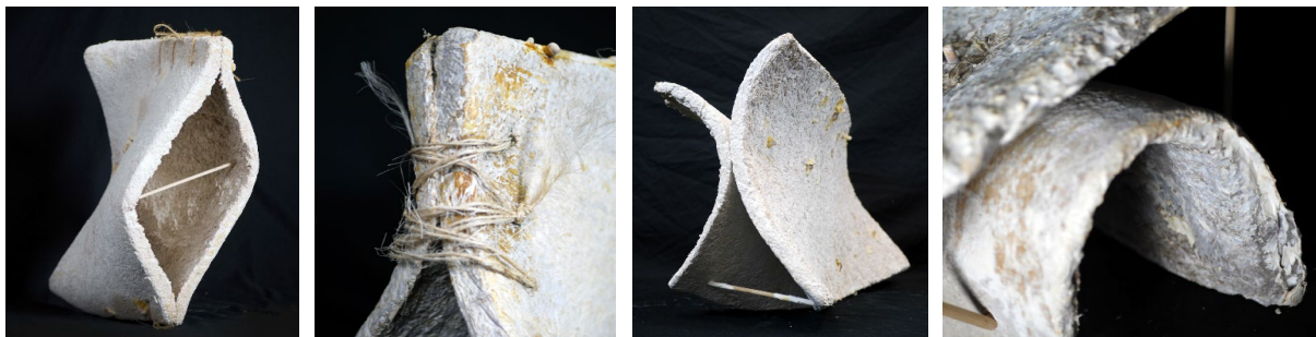
Figure 2. Specimens and details of the active bending myco-sheet improvisations.
