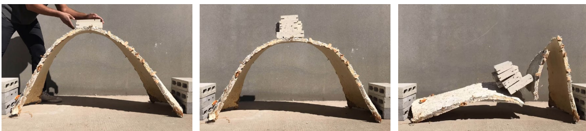
Figure 7. Testing the Unrolled Myco-Arch to failure. The arch, which weighed 3.5 kg held a concentrated load of 31 kg before collapsing.
