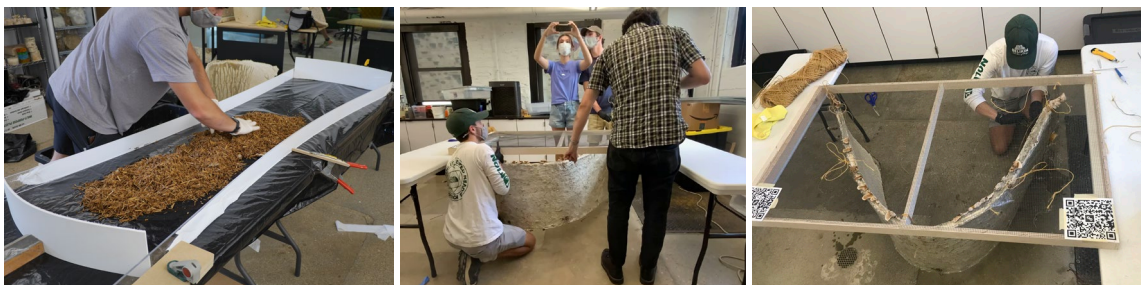
Figure 6. Forming process of myco-materials from loose inoculated hemp substrate (right) to working with smartphone-based augmented reality to register the arch form into the myco-sheet.
