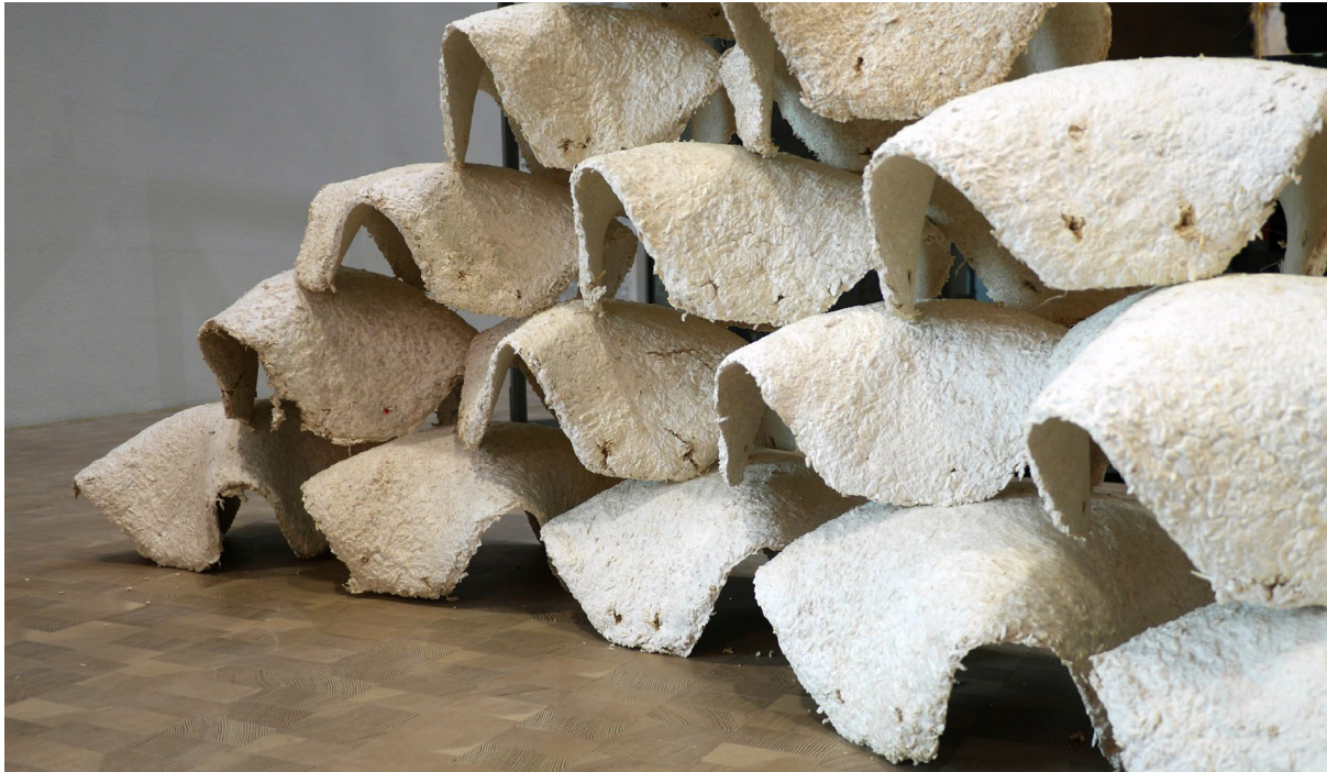
Figure 4. Screen wall structure made with gravity-formed mycelium composite material sheets. The individual units were grown and formed in the MycoMatters Lab by Ann Lomshek and Nicole Reimert Burró, students at Kansas State University.
