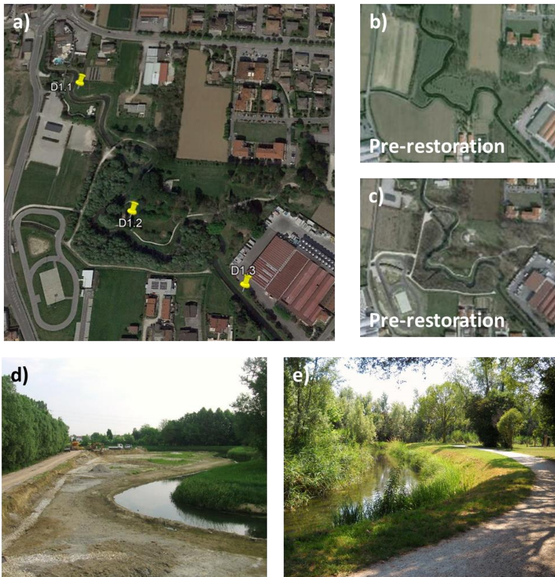
Figure 27. The restored section of the tributary Rio Draganziolo. a) aerial image of the section of the Rio Draganziolo; where restoration occurred; b) pre-restoration; c) post restoration; d) image showing the construction of the two-stage channel and meandering; e) photograph of the site post-restoration.
