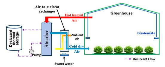
Figure 14. Desiccant greenhouse with use of additional residual heat (daytime operation).
