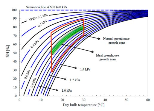
**Figure 1.** Normal and ideal greenhouse growth zones according to vapor pressure deficit levels. Reprinted with permission from Ref. [13]. Copyright 2016 Elsevier.
