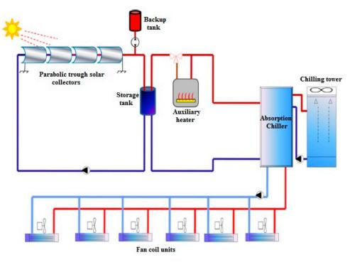
**Figure 4.** An absorption cooling system coupled with parabolic trough solar collectors. Reprinted with permission from Ref. [88]. Copyright 2013 Elsevier.
