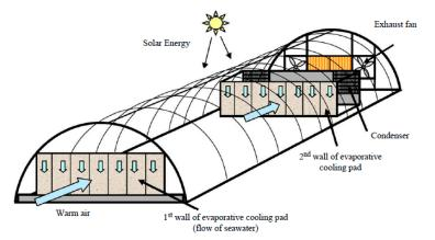
**Figure 9.** Water recovery in the evaporative cooling system of a seawater greenhouse in Oman. Reprinted with permission from Ref. [94]. Copyright 2005 Elsevier.
