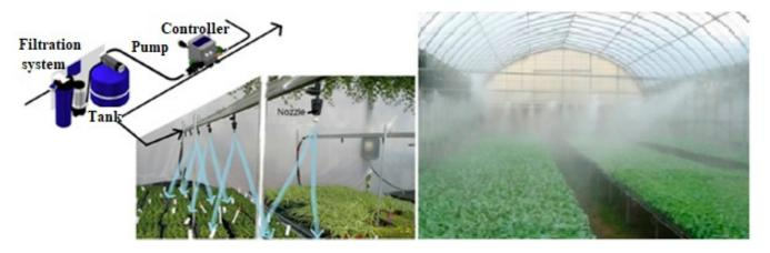
**Figure 7.** Schematic of cooling by a fogging system. Reprinted with permission from Ref. [97]. Copyright 2019 Elsevier.
