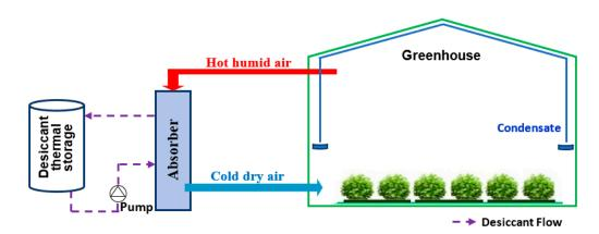
Figure 13. Closed desiccant greenhouse (daytime operation).
