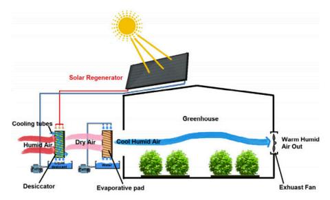
**Figure 8.** Schematic of solar-assisted desiccant cooling system. Reprinted with permission from Ref. [97]. Copyright 2019 Elsevier.
