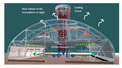
**Figure 12.** Air circulation in the greenhouse cooled by the day-to-night thermal storage system. Adapted from [131].
