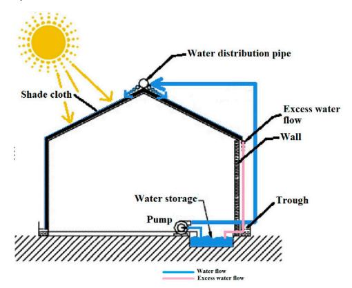
**Figure 6.** Schematic of cooling by roof evaporative system. Reprinted with permission from Ref. [97]. Copyright 2019 Elsevier.
