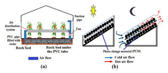
**Figure 11.** Thermal-storage-based systems used in greenhouses: (**a**) rock bed storage; (**b**) PCM storage. Reprinted with permission from Ref. [152]. Copyright 2018 Elsevier.
