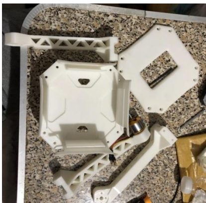
FIGURE 20: 3D printed airframe parts
