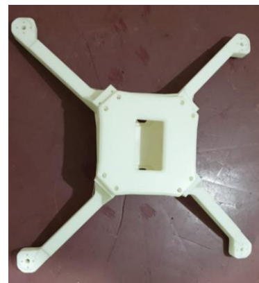
FIGURE 21: Final arrangement of the present X-Quadcopter
