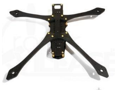
FIGURE 3: Dead Cat-like quadcopter
