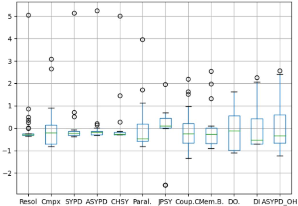
Figure 1. Metric results grouped. ASYPD\_OH (ASYPD overhead) is the extra percentual time comparing the ASYPD (simulation + queues, interruptions, failures...) and useful SYPD, introduced to quantify ASYPD properly for the analysis.
