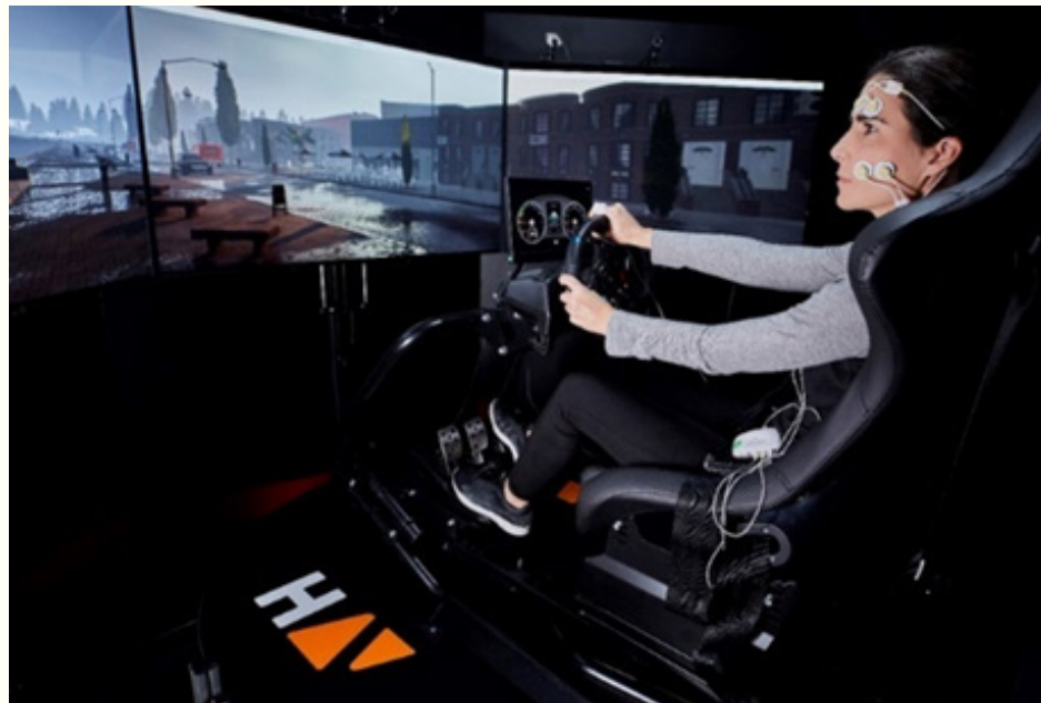
Figure 7. Physiological measurements in the HAV simulator.
