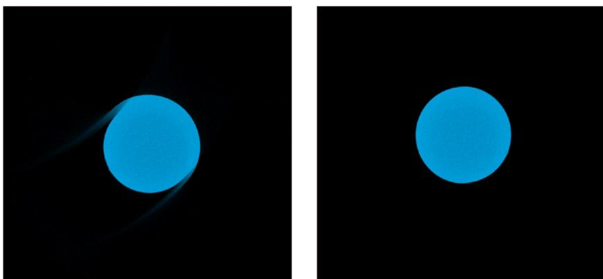
Figure 2: To the left: Horizontal slice with detector misaligned by about 3mm and a helical radius error of about 0.4mm. To the right: Horizontal slice with corrected geometry
