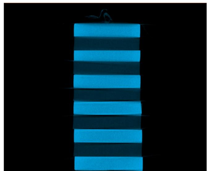
Figure 3: A vertical slice of a stack from a scan of Perspex and aluminium discs alternately stacked, reconstructed by Katsevich's algorithm with slightly wrong vertical detector shift.
