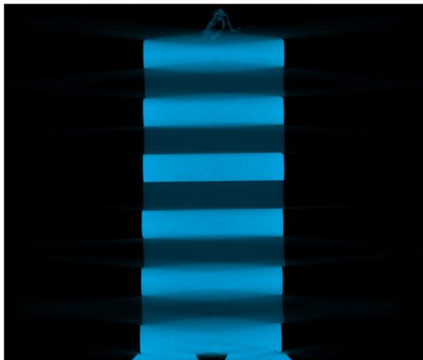
Figure 1: A vertical slice of a stack from a scan of Perspex and aluminium discs alternately stacked, reconstructed with FDK.
