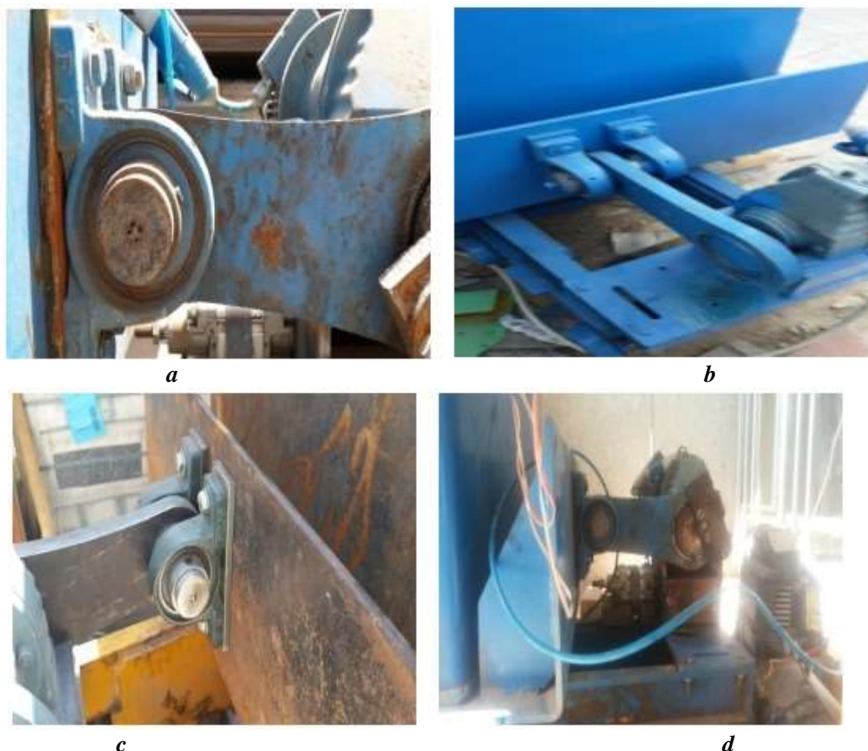
Plate 3: CAMA and pin connected during manufacturing of shaking box.
