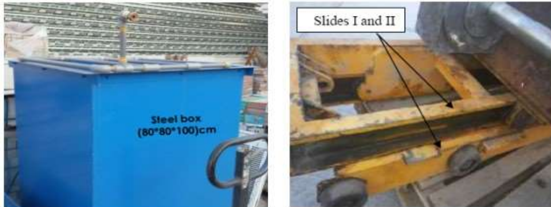
Plate 2: Slides and base bracket system during manufacturing of shake box.
