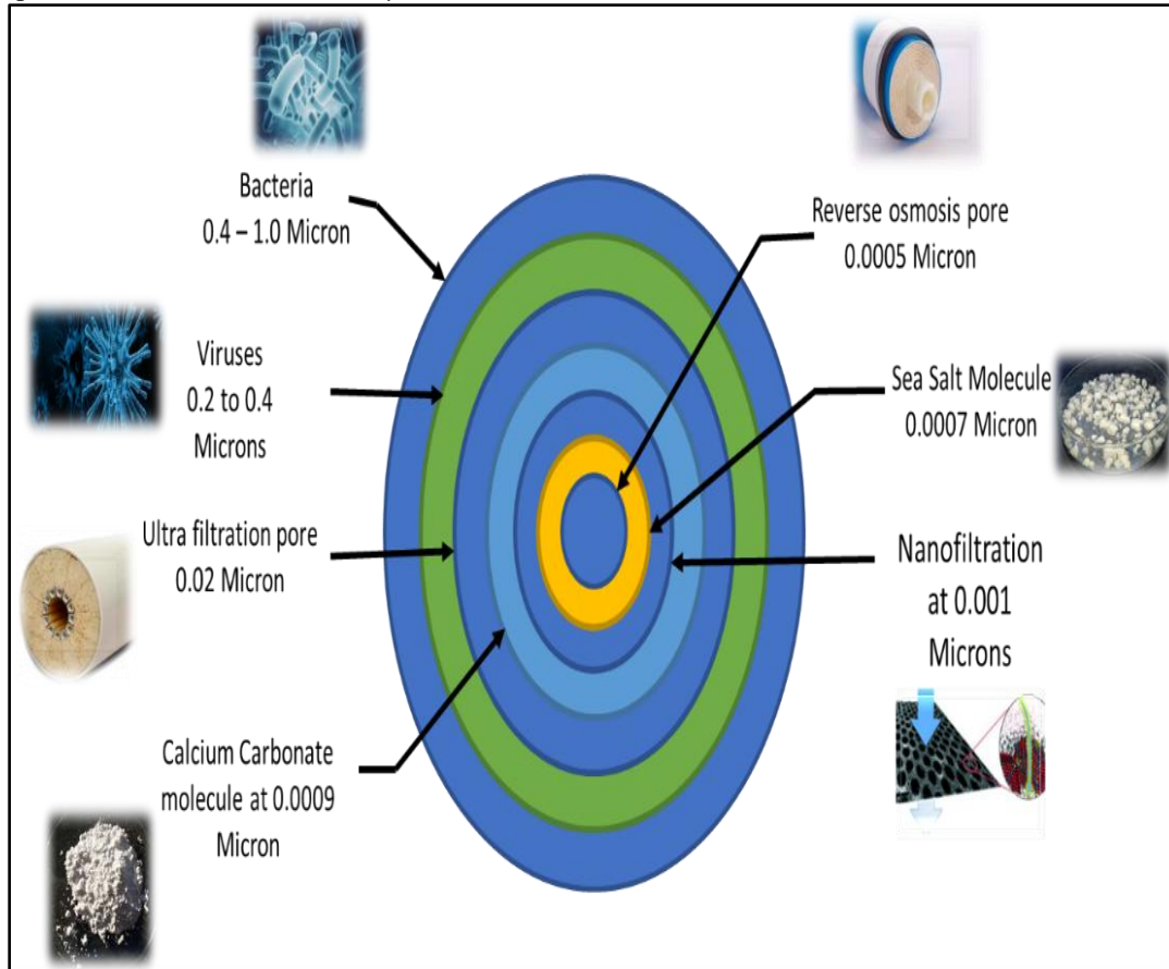
Fig. 1:- Membrane pore size compared with the particle size of foreign matter[6].
