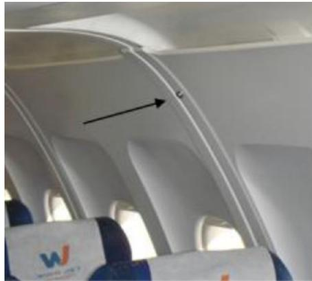
**Position of a temperature/humidity sensor in the cabin** (Giaconia C. et al. (2015), *A correlation linking the predicted mean vote and the mean thermal vote based on an investigation on the human thermal comfort in short-haul domestic flights*, Applied Ergonomics 48, pp. 202-213 [3])
