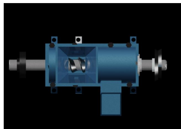
Fig. 3. Screw Fixed Inside The Barrel Ready For Coupling
