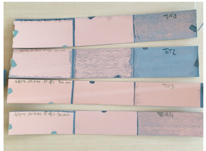
Figure 4: HPCS copper coatings obtained with different spraying conditions. Substrates, made of thermoset CFRC, had, in each column, the same PEEK PPF thickness (300 \mu\text{m} on the left, 50 \mu\text{m} on the middle and 25 \mu\text{m} on the right).
