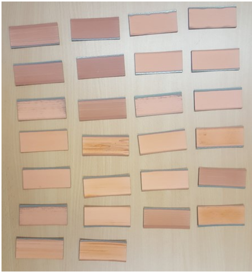
Figure 5: photographic image of Cu HPCS onto thermoset CFRC with PPF, with different spraying parameters (temperature, pressure and stand-off distance).
