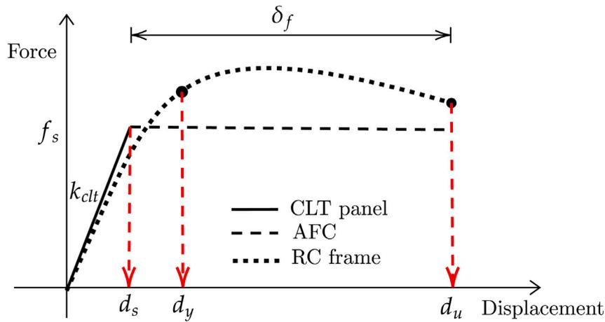
Fig. 3. Qualitative explanation of the design problem:  $k_{clt}$  is the in-plane stiffness of the CLT wall,  $d_y$  and  $d_u$  are the yield and ultimate displacements of the RC frame,  $d_s$  is the slip displacement of the AFC, and  $\delta_f$  is the displacement interval corresponding to the AFC activation.
