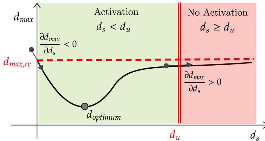
Fig. 4. Qualitative illustration of the trend of the maximum displacement  $d_{max}$  as a function of the damper slip displacement  $d_s$ . (For interpretation of the references to colour in this figure legend, the reader is referred to the web version of this article.)
