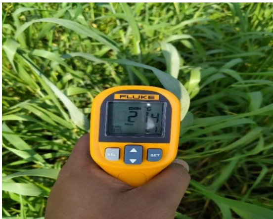
Plate No 3: Infrared Thermometer to measure Canopy Temperature.
