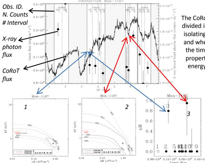
The CoRoT light curves are divided into time intervals isolating dips and bursts, and where we estimated the time resolved X-ray properties (photon and energy fluxes,  $N_H$ ,  $kT$ , etc.)
