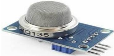
Fig. 1. MQ-135 Gas Sensor.
