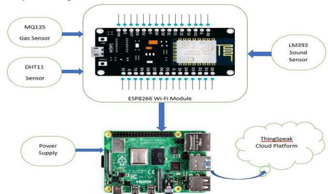
Fig. 6. System Architecture.
