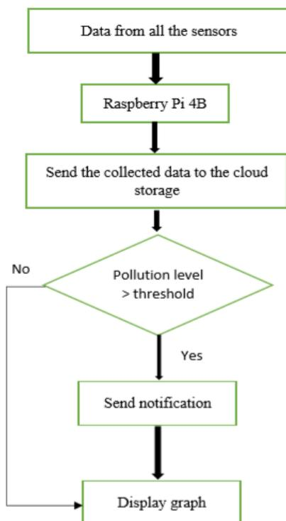
Fig. 8. Flow of data within the system.
