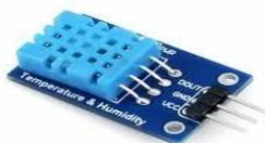
Fig. 3. DHT11 Humidity and Temperature sensor.
