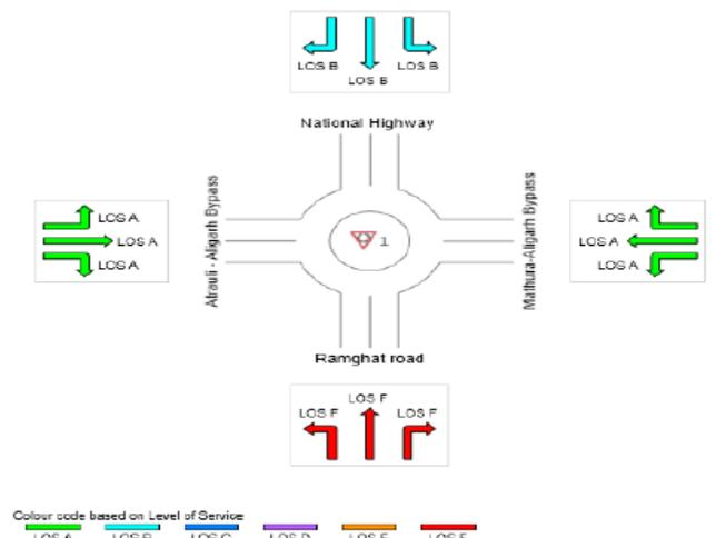
**Figure 3 (b): Capacity Scheming of 3-leg Intersection in SIDRA (Veh/hr/Movement)**
