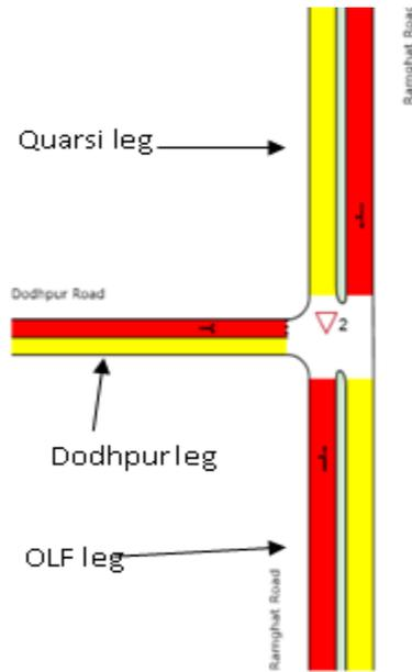
**Figure 2 (b): 3-Leg Intersection Layout in SIDRA**
