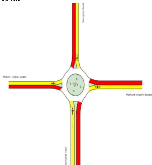
**Figure 2 (a): Roundabout Layout in SIDRA**
