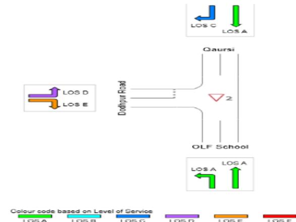
**Figure 4 (a): Level of Service of Roundabout (per Leg per Movement)**
