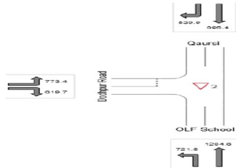
**Figure 3 (a): Capacity Scheming of Roundabout in SIDRA (Veh/hr/Movement)**
