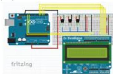
**Fig. 4. Schematic of the complete assembly of the Prototype.**
