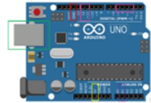
**Fig. 3. Representation of the applicable Arduino Uno Board.**
