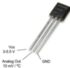
**Fig. 2. LM35 temperature sensor.**
