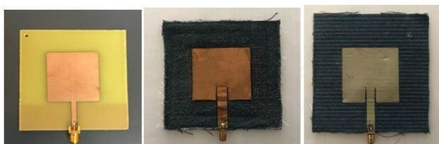
Fig. 2 Antennas (a) Non textile (b) Semi textile (c) Fully textile.
