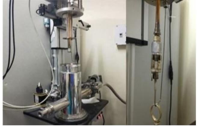
**Fig.1 Measurement of fabric properties on dielectric Broadband spectrometer**
