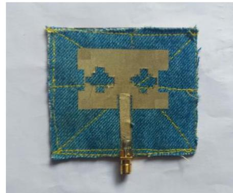
**Fig. 6 Demonstrated modified geometry of revised wearable fully textile antenna.**
