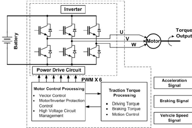
Fig. 1. Components of a typical electric vehicle propulsion system.
