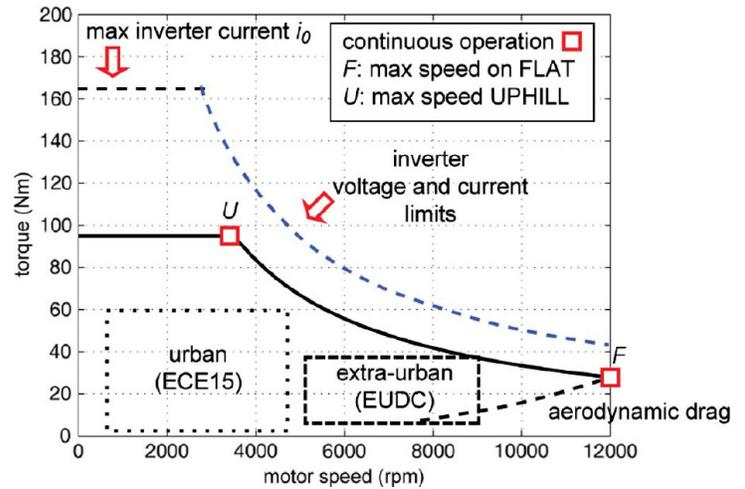
Fig. 2. Sample target description of  $i_0$  torque for an electric vehicles.
