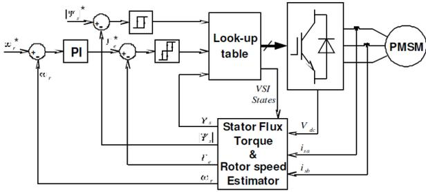
Fig. 5. DTC control scheme for PMSM.
