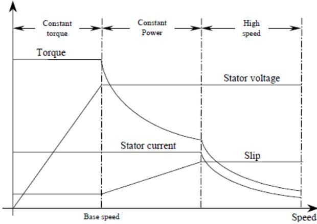
Fig. 3. Induction motor characteristics.
