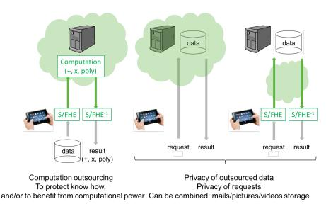
Fig. 1. A need for processing encrypted data, to ensure privacy in outsourced computation, outsourced
