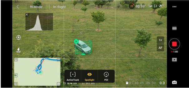
Fig. 5. Graphical interface of the DJI Fly application, which allows you to mark an object for tracking with the marked tracking options Activetrack - Spotlight- point of interest. Source: own source
