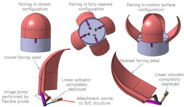
Fig. 5. Concept of aerodynamic control surface mechanism for RETALT 2
