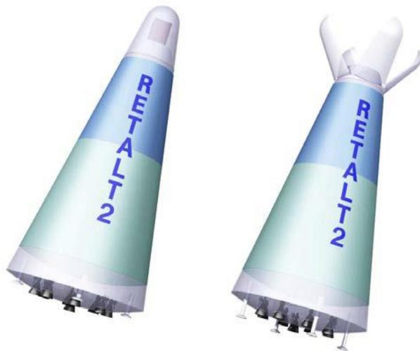
Fig. 2. Conceptual sketch of the RETALT2 spacecraft. Configurations from left to right: launch, descent and landing.
