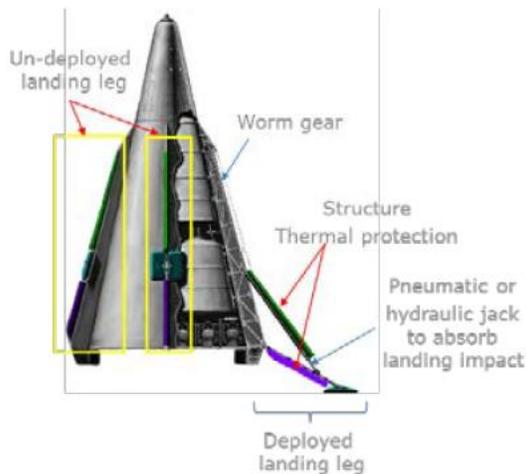
Fig. 7. RETALT 2: deployment kinematics
