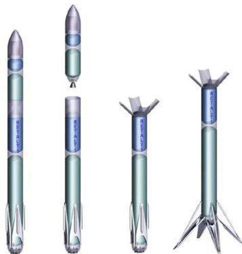
Fig. 1. Conceptual sketch of the RETALT1 spacecraft. Configurations from left to right: launch, stage separation, first stage descent, first stage landing.
