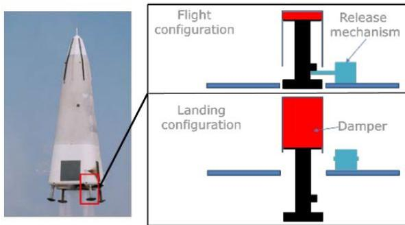
Fig. 6. RETALT 2: pneumatic cylinder
