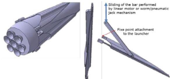
Fig. 3. RETALT1: linear actuator attached to sliding bar
