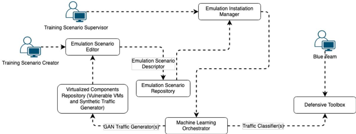
Figure 3: Extract from the SPIDER high-level reference architecture.
