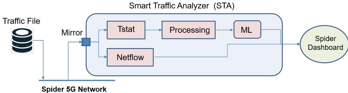
Figure 2: Smart Traffic Analyzer (STA) internal components
