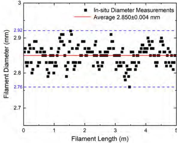
Figure 4: Oscillations of the filament diameter along the filament during precision extrusion of a PLA/5% Mg composite.
