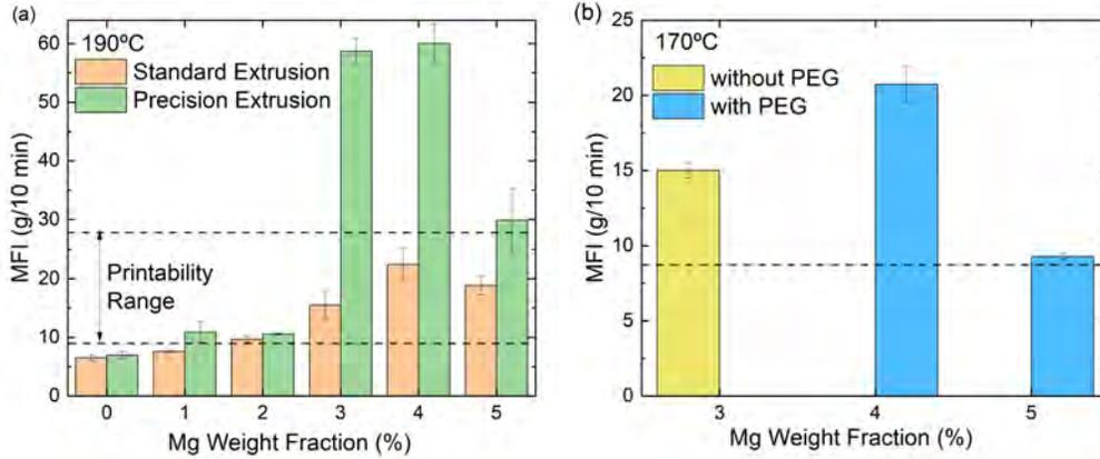
Figure 8: (a) MFI at 190°C of standard extruded and precision extruded PLA/Mg filaments as a function of the Mg content. (b) MFI at 170°C of precision extruded filaments of PLA/Mg and PLA/Mg/5%PEG as a function of the Mg content. The MFI range for printability is marked by the horizontal dashed lines.
