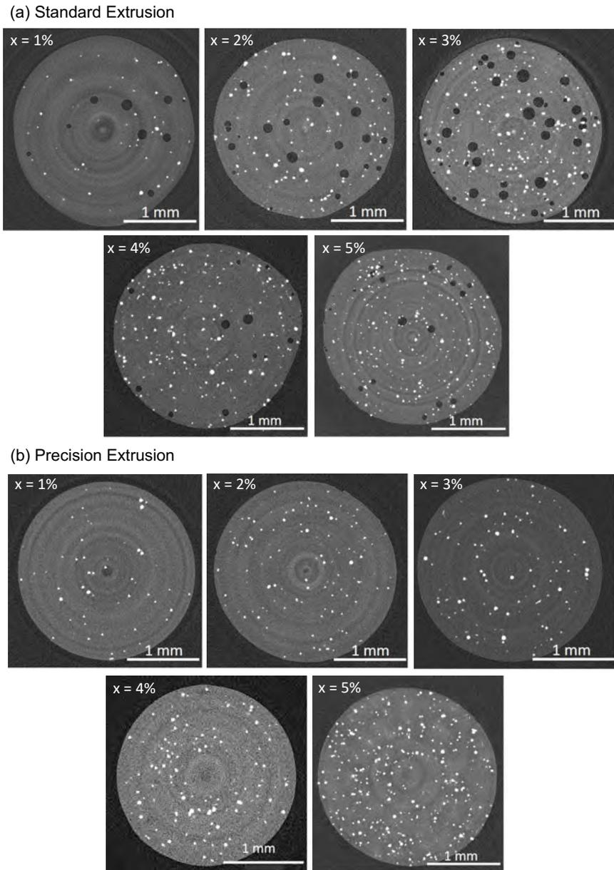
Figure 3: Representative cross sections obtained by X- $\mu$ CT of PLA/Mg filaments after (a) standard extrusion and (b) precision extrusion.  $x$  stands for the weight fraction of Mg. Filament diameter was 2.85 mm in all cases.
