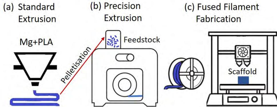
Figure 1: Schematic of the manufacturing process from the PLA and Mg powders to the fabrication of scaffolds by FFF. (a) Thermal mixing of raw materials (PLA and Mg powders) at 180°C, followed by extrusion. (b) Pellets of the extruded filaments were extruded again in a filament maker machine. (c) Extruded filaments were spooled and scaffolds were manufactured by FFF.
