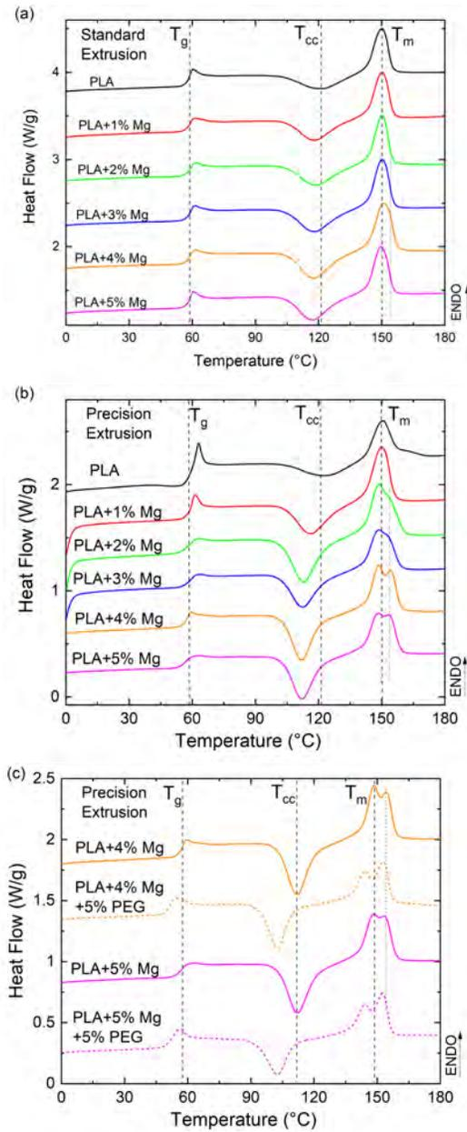
Figure 5: Heat flow curves of PLA/Mg filaments during DSC at a heating rate of 10°C/min. (a) After standard extrusion. (b) After precision extrusion. (c) Effect of PEG on the heat flow of PLA/Mg filaments. Glass transition temperature ( $T_g$ ), cold crystallization temperature ( $T_{cc}$ ), and melting point ( $T_m$ ) are indicated with dashed lines.
