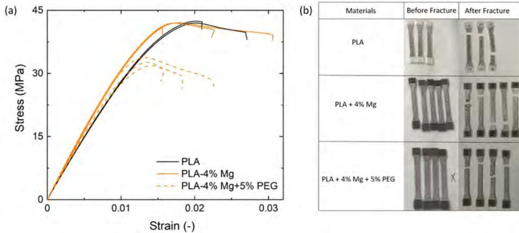
Figure 9: (a) Tensile stress-strain curves of dog-bone specimens of pure PLA, PLA-4% Mg and PLA-4% Mg with 5% PEG deformed parallel to the printing direction. (b) Images of the specimens after fracture.
