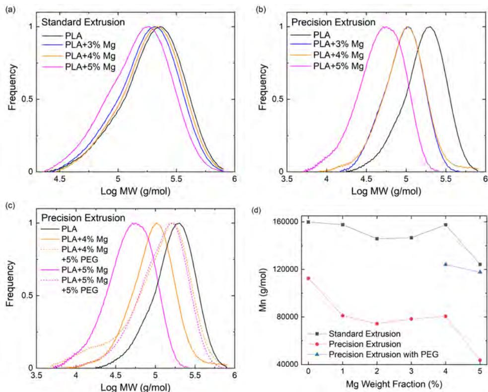
Figure 7: Molecular weight distributions of PLA/Mg composites. (a) After standard extrusion. (b) After precision extrusion. (c) Effect of PEG on the molecular weight distribution after precision extrusion. (d) Evolution of the average molecular weight with Mg content after standard and precision extrusion.
