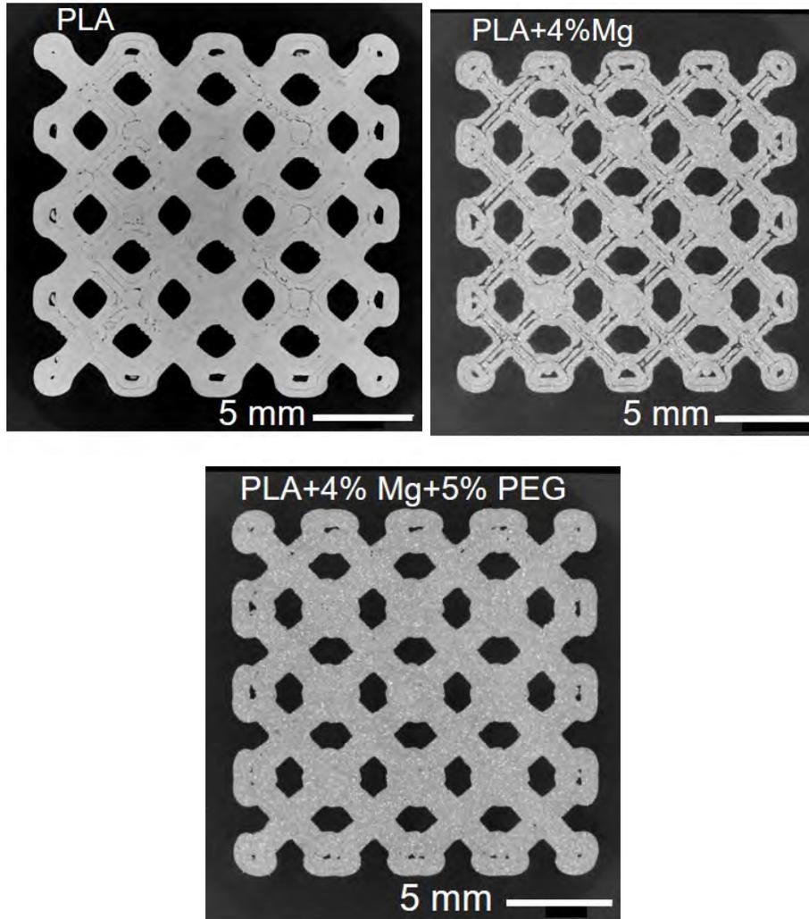
Figure 10: Cross-sections fcc scaffolds extracted from the tomograms obtained by X- $\mu$ CT. (a) PLA. (b) PLA/4% Mg. (c) PLA/4% Mg/5% PEG.
