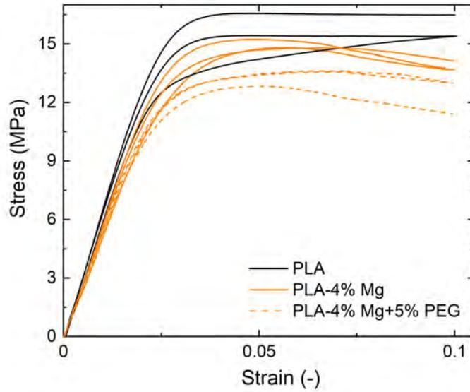
Figure 11: Experimental engineering stress-strain curves in compression of fcc scaffolds.
