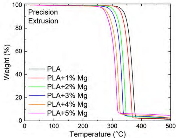
Figure 6: Weight loss as a function of temperature obtained from TGA for the precision extruded composite containing different weight fractions of Mg particles.
